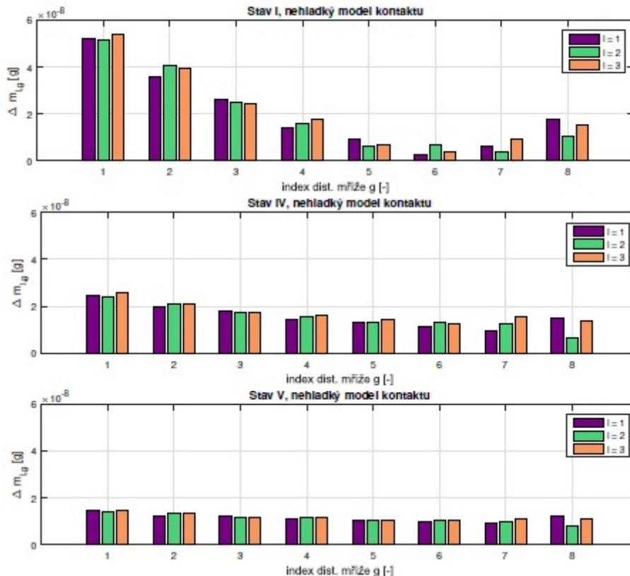
Fig. 7: Fretting wear per one hour as the function of the spacer grids in states I, IV and V.
