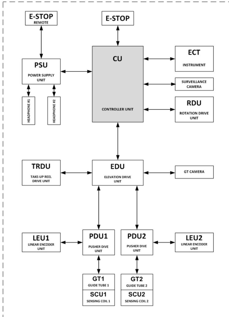
Figure 2. – Control System Block Scheme (with EC module installed)
