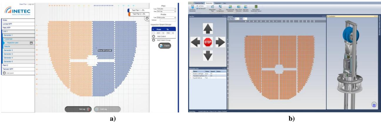
Figure 7. EddyOne inspection management software (a) and EddyOne manipulator control software (b)
